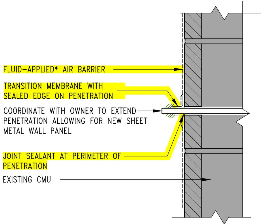
\*AIR BARRIER MEMBRANE MAYBE FLUID-APPLIED OR SELF-ADHERING.
