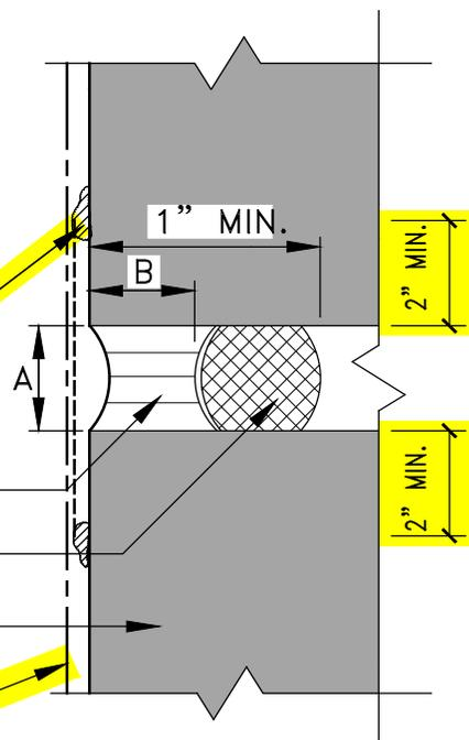
\*AIR BARRIER MEMBRANE MAYBE FLUID-APPLIED OR SELF-ADHERING.
