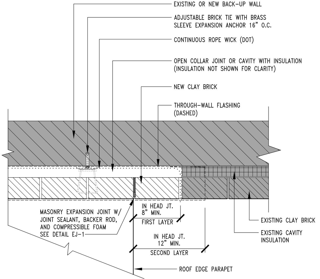
NOTE: FOR NEW CONSTRUCTION, SHOW JOINT REINFORCEMENT W/ADJUSTABLE TIES AND AIR BARRIER.
