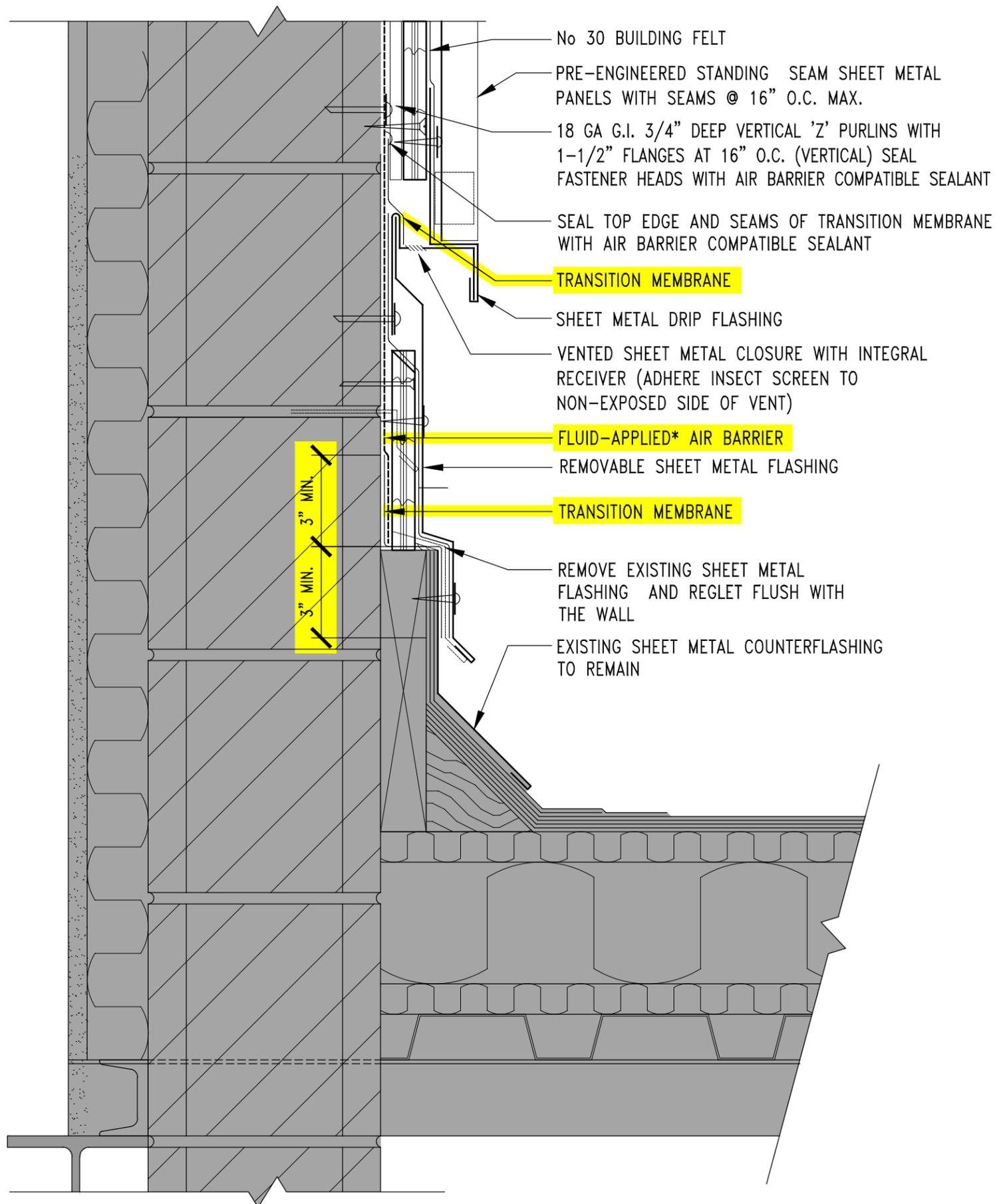
\*AIR BARRIER MEMBRANE MAYBE FLUID-APPLIED OR SELF-ADHERING.
