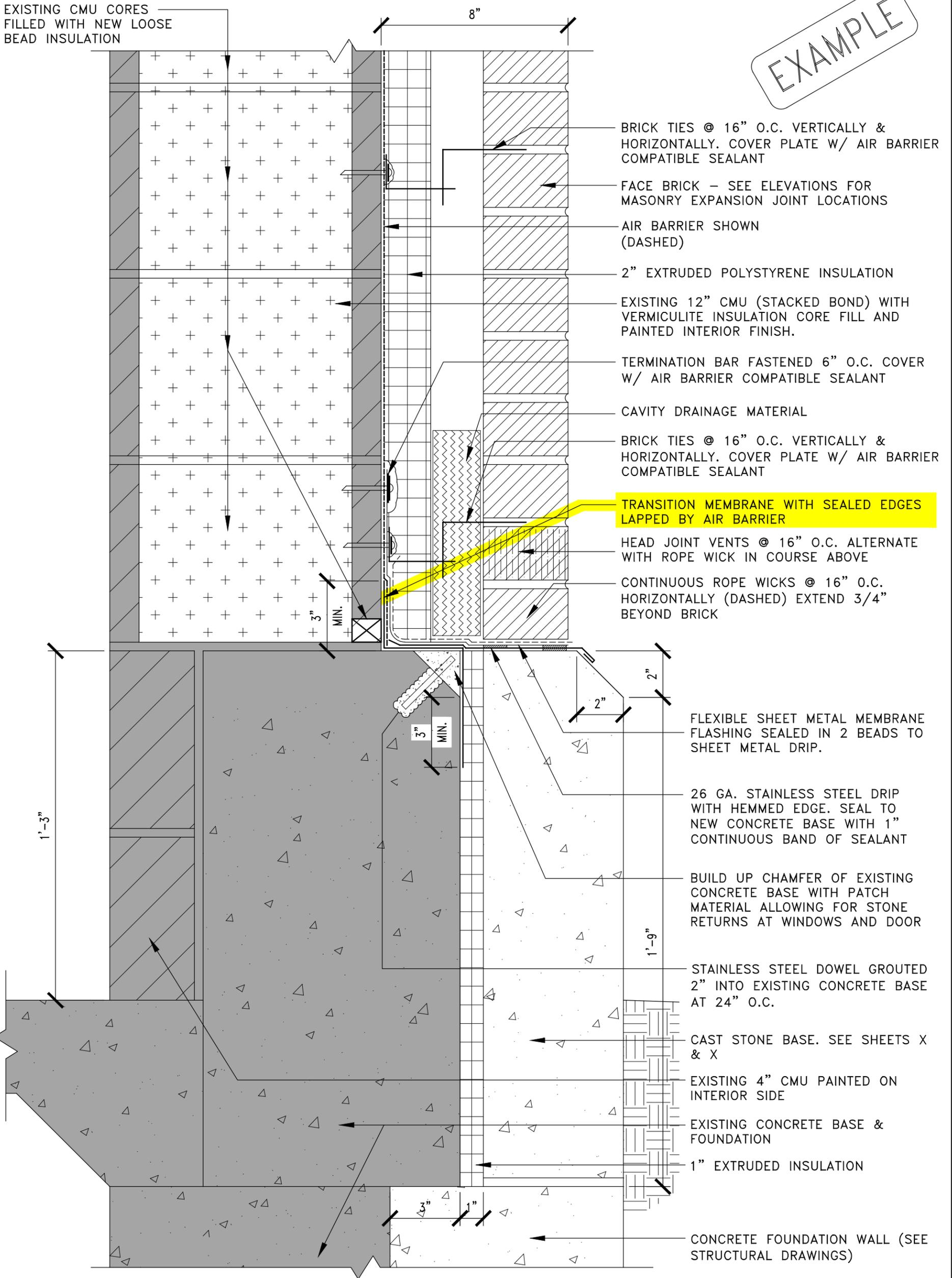
BRICK TIES @ 16" O.C. VERTICALLY & HORIZONTALLY. COVER PLATE W/ AIR BARRIER COMPATIBLE SEALANT
