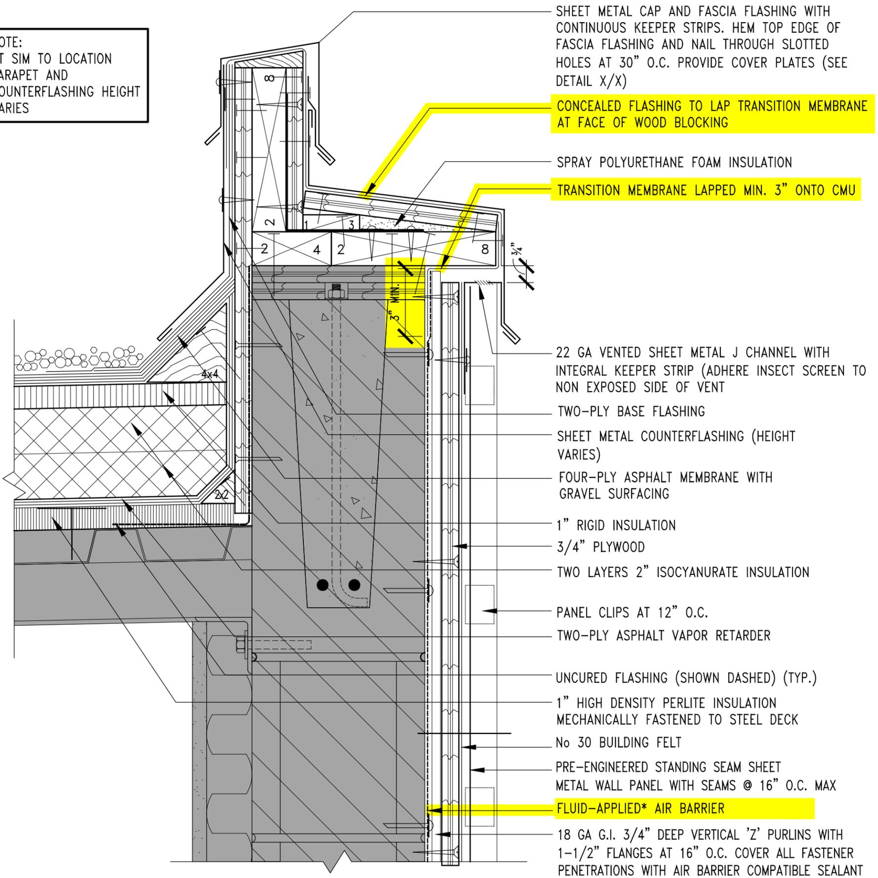
SHEET METAL CAP AND FASCIA FLASHING WITH CONTINUOUS KEEPER STRIPS. HEM TOP EDGE OF FASCIA FLASHING AND NAIL THROUGH SLOTTED HOLES AT 30" O.C. PROVIDE COVER PLATES (SEE DETAIL X/X)
