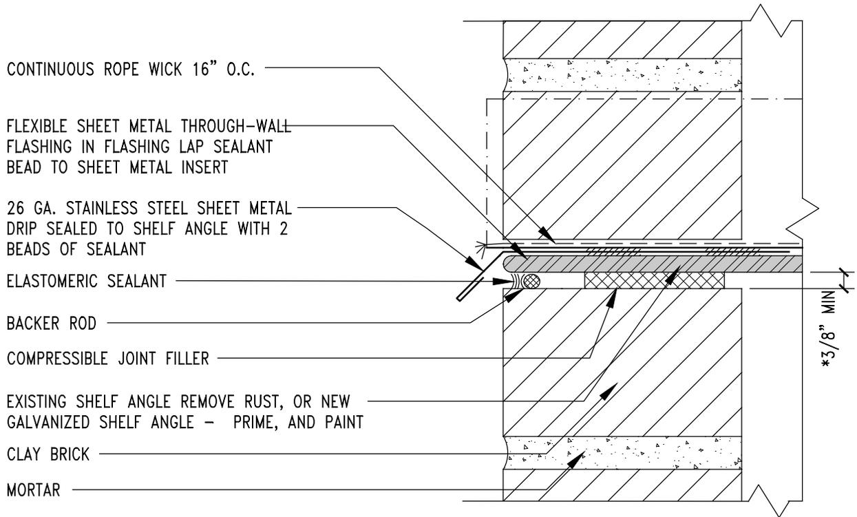
NOTE: A/E TO VERIFY SIZE OF HORIZONTAL EXPANSION JOINT BASED ON CALCULATIONS FOR EXPANSION OF THE BRICK AND DEFLECTION OF THE SHELF ANGLE.
