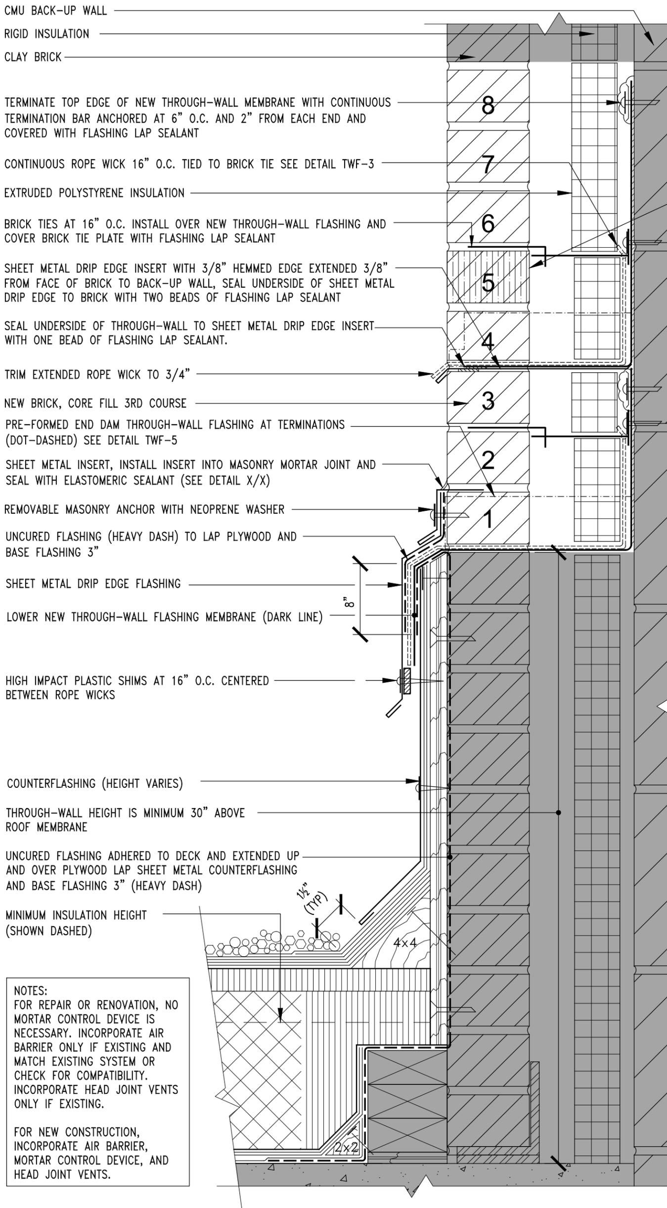
IN NEW CONSTRUCTION, INSERT HEAD JOINT VENT IN ALTERNATING HEAD JOINT FROM ROPE WICKS, ONE COURSE ABOVE
