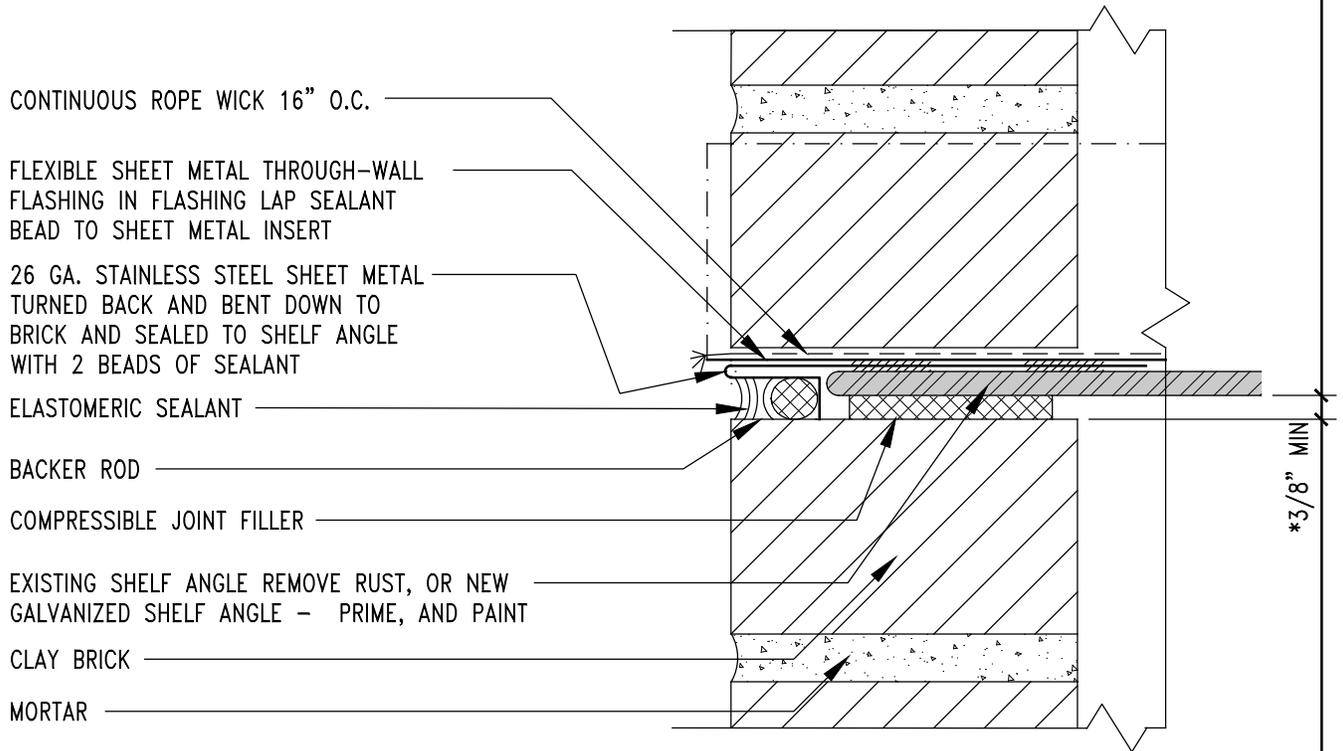
NOTE: A/E TO VERIFY SIZE OF HORIZONTAL EXPANSION JOINT BASED ON CALCULATIONS FOR EXPANSION OF THE BRICK AND DEFLECTION OF THE SHELF ANGLE.
